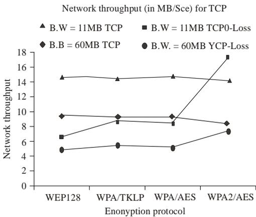
Fig. 1: Network throughputs for TCP protocol
